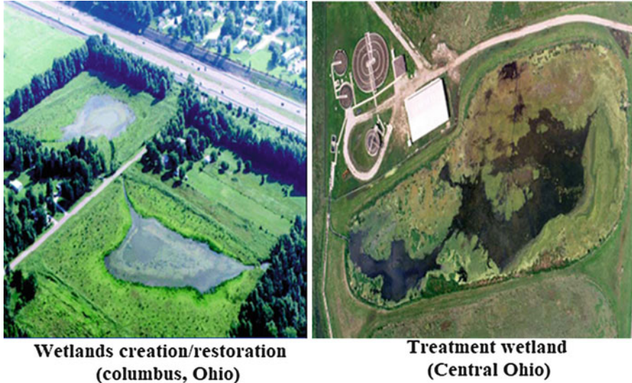
Fig. 5.13 Wastewater treatment via constructed wetlands. (ITRC 2009)
