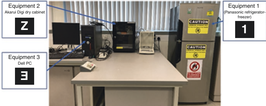
Fig. 6.3 Small-scale workcell with various equipment and their respective marker designs
