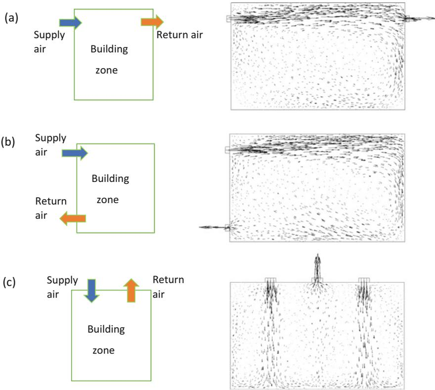
**Fig. 10.3** Examples of mixing ventilation systems (left) and the corresponding airflow pattern (right): (a) opposite side walls supply (high) and extract (high), (b) one side wall supply (high) and extract (low), and (c) ceiling supply and extract
