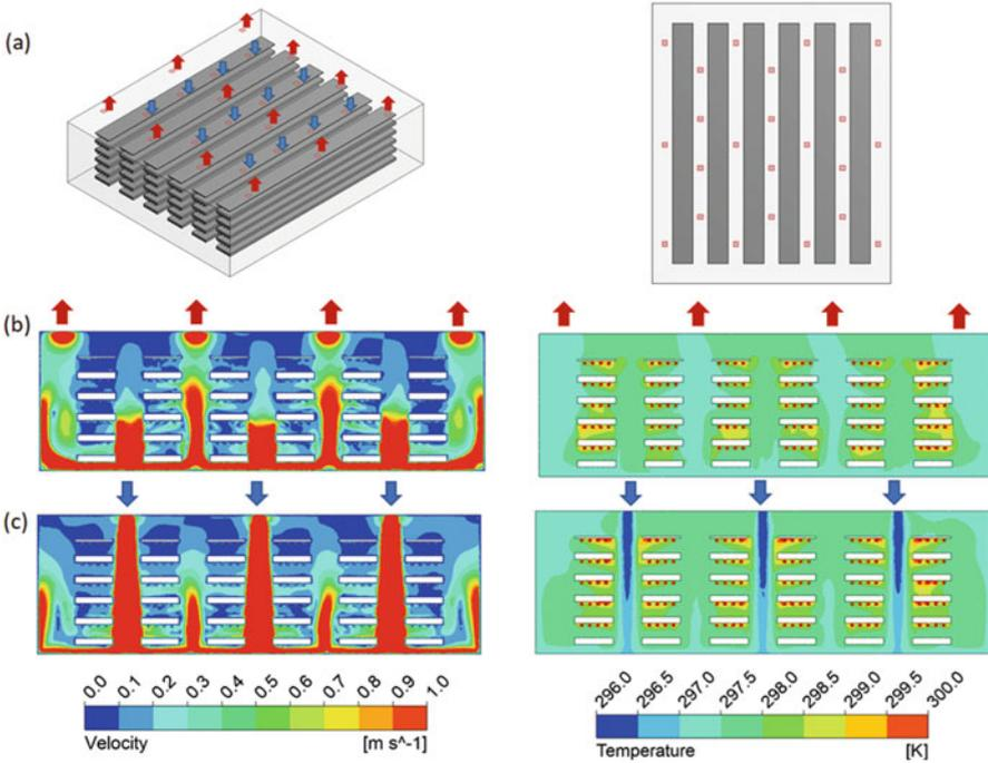
**Fig. 10.4** An example of air ventilation system with ceiling supply and extract vents (Zhang and Kacira 2017): (a) the layout of the supply and extract vents, (b) the air velocity and temperature distribution at outlet vents, and (c) the air velocity and temperature distribution at inlet vents. The analysis and results on air velocity and temperature distributions were obtained using computational fluid dynamics modeling
