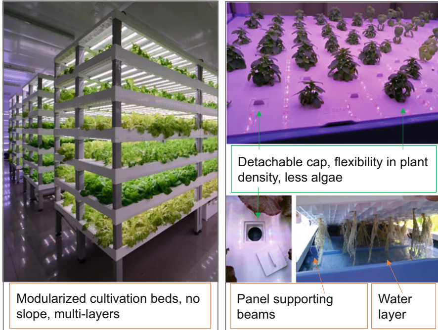
Fig. 3.3 Images of the modified hybrid hydroponic system in a plant factory (Photos provided by Fujian Sanan Sino-Science Photobiotech Co., Ltd)
