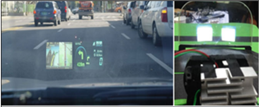
Fig. 4 A back light unit and system design of the HUD using dual panels and LEDs for a multi windows
