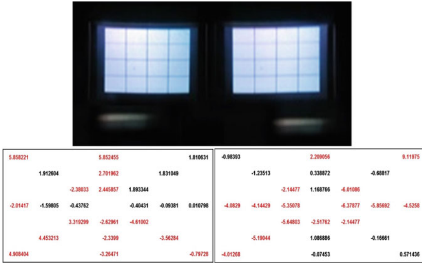
Fig. 5 A distortion analysis of dual projected image in the HUD using the combiner lens
