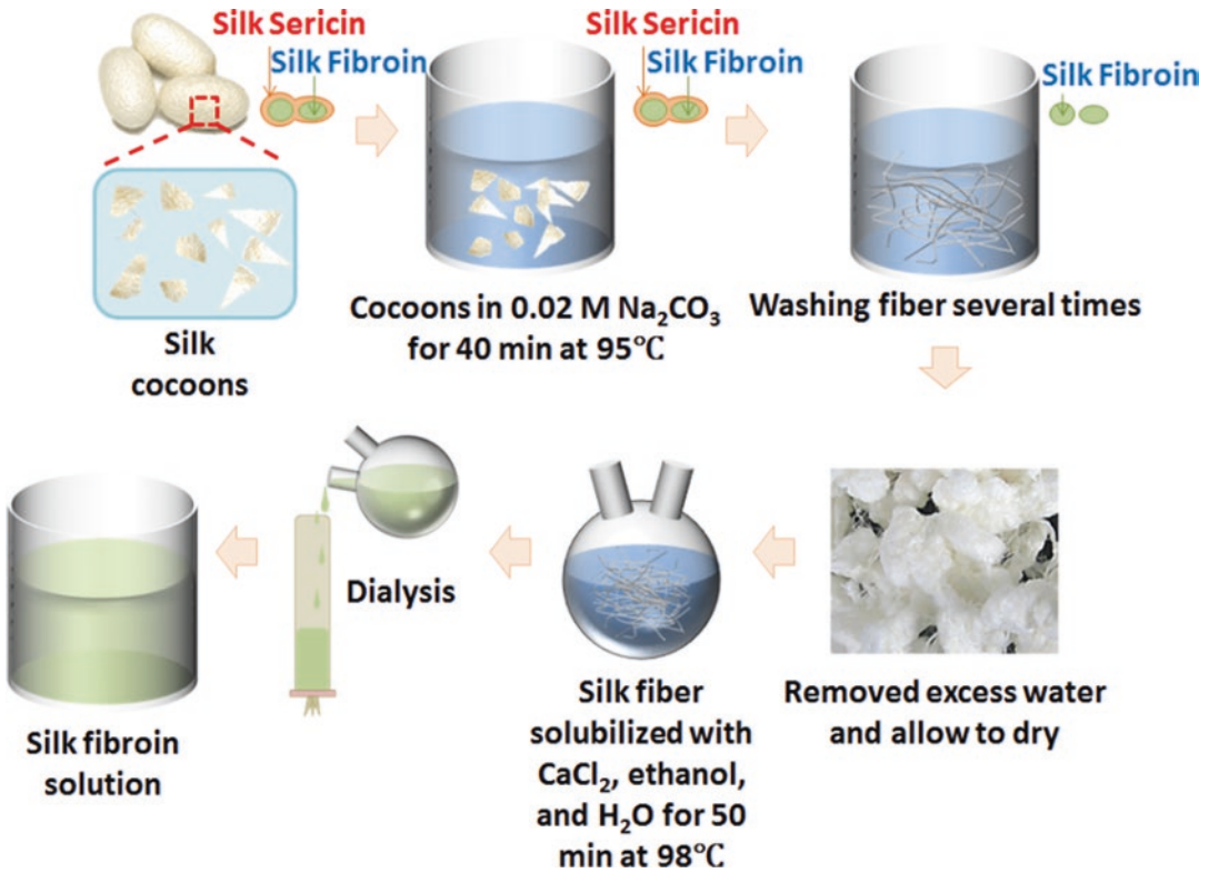
Fig. 7.1 Schematic of SF extraction procedure. Silk cocoon was degummed with an aqueous solution of 0.02 M Na 2 CO 3 by boiling for 40 min at 95 °C, and then washed with distilled water to eliminate the glue-like sericin pro-
