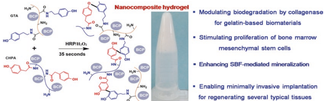
Fig. 13.4 Horseradish peroxidase-mediated fabrication of chitosan/gelatin and BCP nanoparticles-based nanocomposite hydrogel for born tissue regeneration
