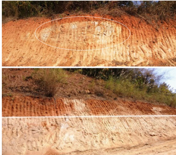
Fig. 1 IITG cut slope site depicting two layers of soil and weathered corestones (top layer is referred as soil 1 while the bottom layer as soil 2)
