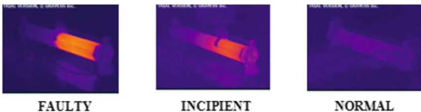
Fig. 3 Different classes of thermal images of rheostat
