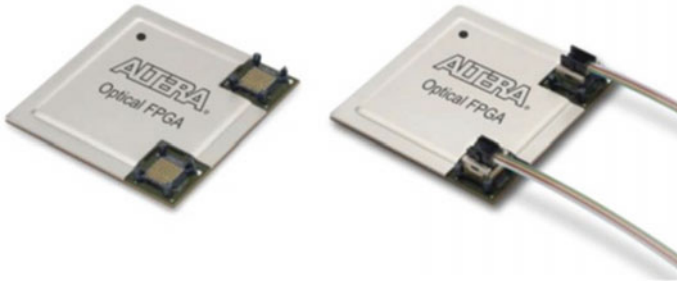
Fig. 8.17 Appearances of 0.7424-mm pitch LGA sockets mounted on Stratix IV package (left) with MicroPOD optical modules (Avago Technologies Ltd.) (right)
