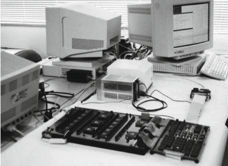
Fig. 1.10 A rapid prototype using 12 FPGAs
