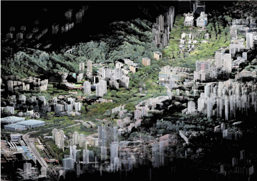
Fig. 17.2 Axonometric projection of a point-cloud model along the Rail Corridor in Tanjong Pagar, Singapore; Credit to —Philipp Urech
