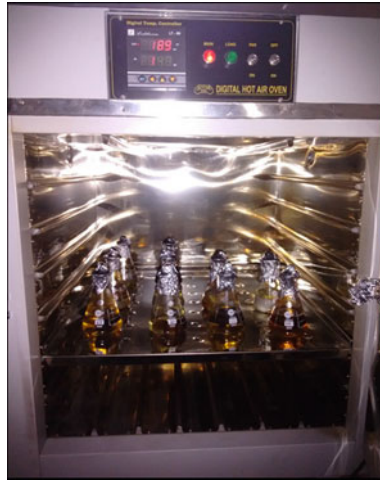
Fig. 1 Samples placed in an air-circulated temperature oven
