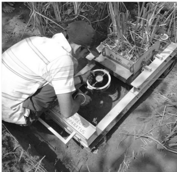
Fig. 1 Schematic diagram of in situ direct shear test apparatus
