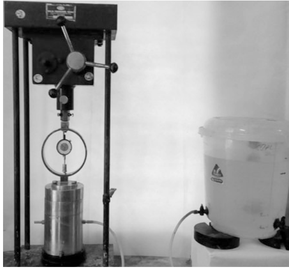
Fig. 2 Transmissivity test apparatus
