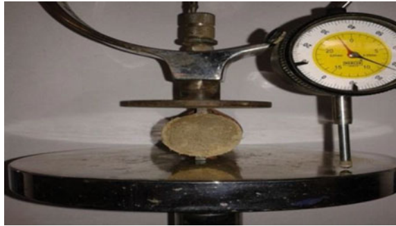
Fig. 1 Photographic view of split-tensile test
