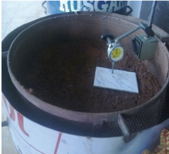
Fig. 2 Heave measurement of pavement
