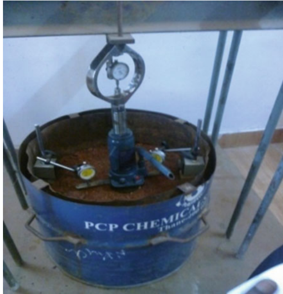
Fig. 3 Cyclic plate load test setup
