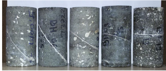
Fig. 3 Jointed rock samples with weak gouge material (kaolin clay)
