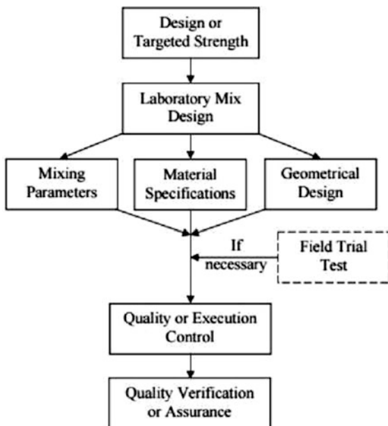
Fig. 7 Typical QA/QC procedure (modified after Coastal Development Institute of Technology 2002 and Usui 2005)
