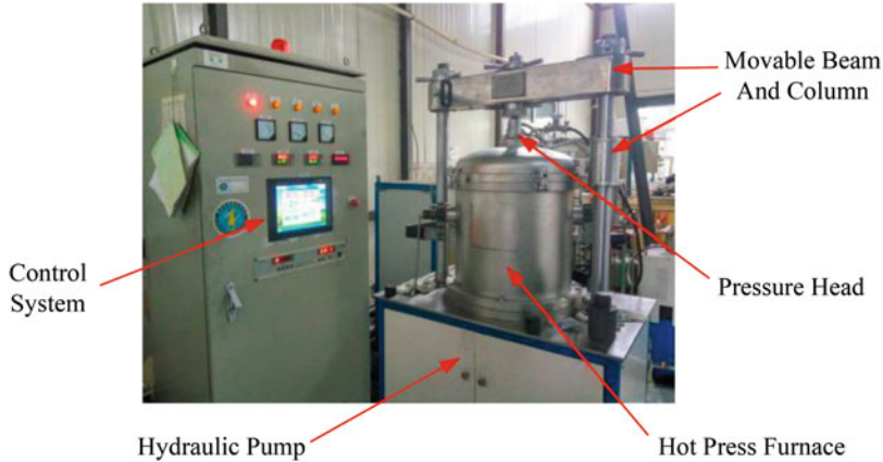
Fig. 28 The temperature-pressure integrated controllable loading vacuum hot-pressing furnace (Li et al. 2017)
