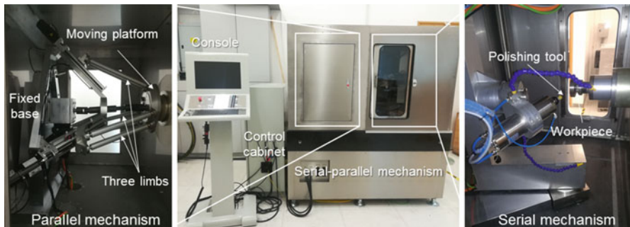
Fig. 21 Prototype of the hybrid serial-parallel polishing machine
