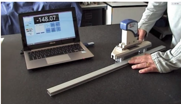
Fig. 33 Talyvel 6 precision electronic level. (Courtesy of Taylor-Hobson plc)
