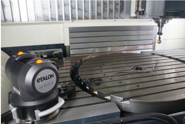
Fig. 44 Calibrate a machine tool with an eTALON LaserTRACER-NG. Measuring uncertainty for spatial displacement (95%) is 0.2 \mu\text{m} + 0.3 \mu\text{m}/\text{m} , and resolution reaches 0.001 \mu\text{m} . (Courtesy of Etalon AG)
