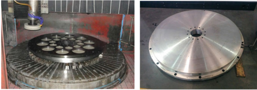
(a)Upper static pressure plate grinding (b) upper static pressure plate surface after grinding
