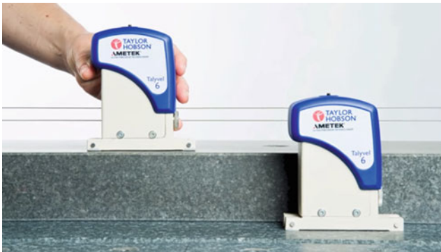
Fig. 32 Two Talyvel Clinometers measure the actual difference in the inclination of two surfaces. (Courtesy of Taylor-Hobson plc)
