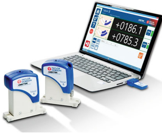
Fig. 30 The Taylor Hobson Talyvel 6 precision digital clinometer offers a larger measuring range ( \pm 45^\circ ), accuracy of within 2 min of arc, and a resolution of 0.01^\circ (in certain display settings 4 s of arc or 0.02 mm/m). (Courtesy of Taylor-Hobson plc)
