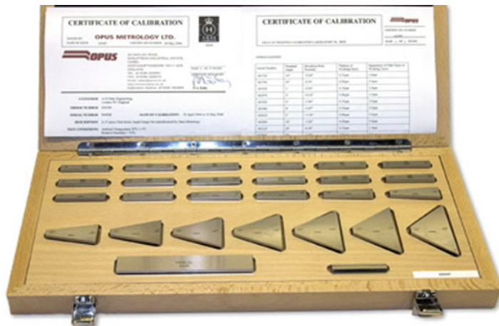
Fig. 15 A typical 27-piece combination angle gauge set. (Courtesy of Thomas Salvesen Enterprises Ltd)
