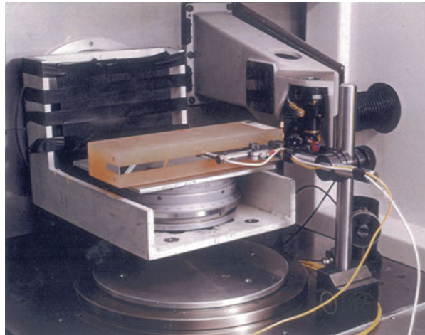
Fig. 8 “Zerodur™” straightedge and proximity sensor can be utilized to calibrate a nanocenter’s X-axis to a very high level of accuracy/precision, in a temperature-controlled machining environment. (Courtesy of Cranfield Precision/Atomic Weapons Establishment, Aldermaston)
