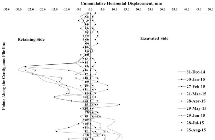
Fig. 3 Horizontal displacement at top of contiguous pile along south side of the plot
