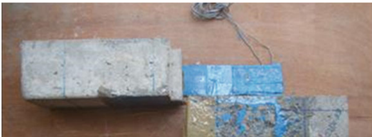
Fig. 4 Failure in CFRP-bonded specimens (50-100-C)
