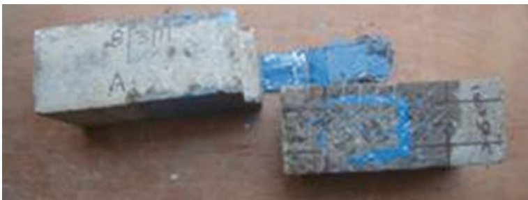
Fig. 5 Failure in GFRP-bonded specimens (50-100-G)
