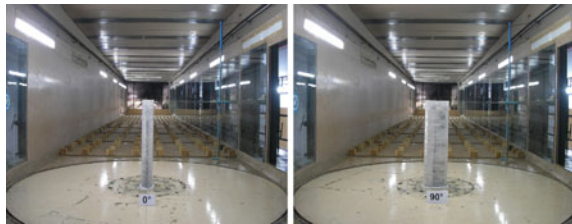
Fig. 3 Elliptic tall building model kept inside the wind tunnel for \theta = 0^\circ and 90^\circ under suburban terrain
