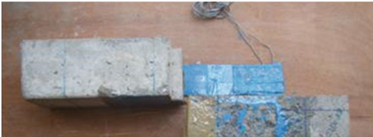
Fig. 4 Failure in CFRP-bonded specimens (50-100-C)
