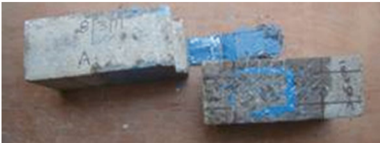
Fig. 5 Failure in GFRP-bonded specimens (50-100-G)
