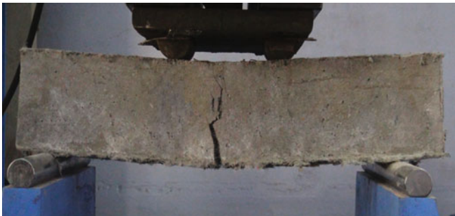
Fig. 8 Failure of ECC prism during four point bending test
