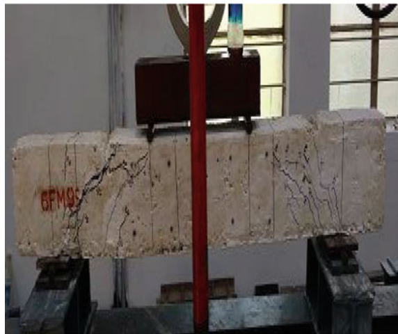
Typical crack pattern of shear beam with fibres -6M9
