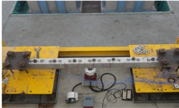
Fig. 7 Experimental setup for the verification of the proposed damage diagnostic algorithm
