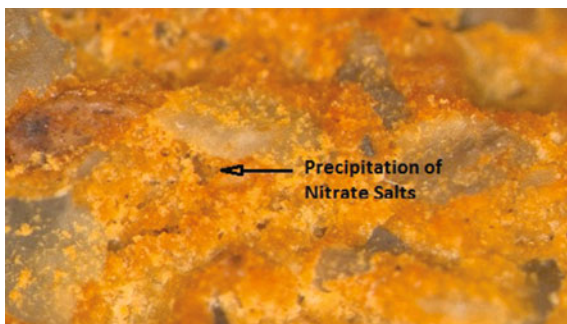
Fig. 6 Stereo microscopic image for BDM particle after 7-day immersion in nitric acid (5% v/v) solution at 2.5× magnification
