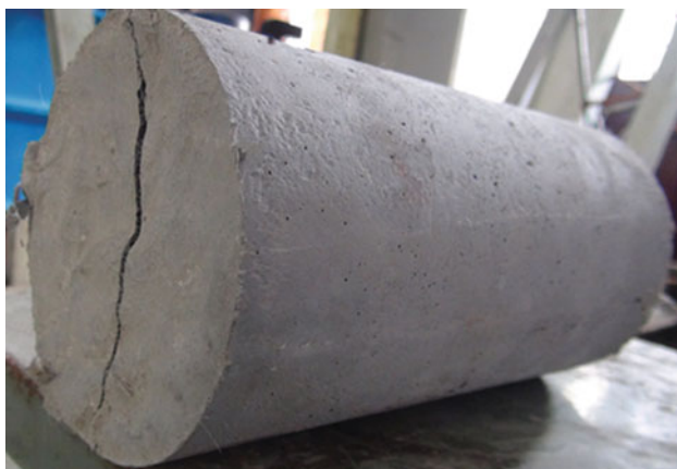
Fig. 4 Failure pattern of cylindrical specimen after split tensile strength test
