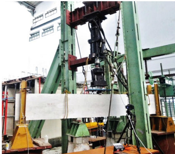
Fig. 2 Monotonic test set-up
