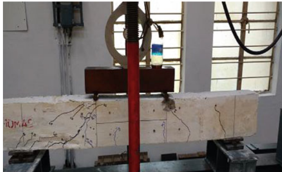
Typical crack pattern of shear beam without fibres - 10M4
