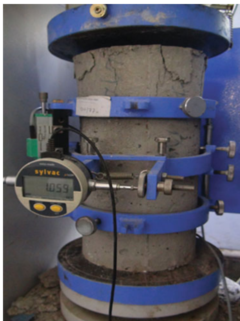
Fig. 3 Failure pattern of cylindrical specimen
