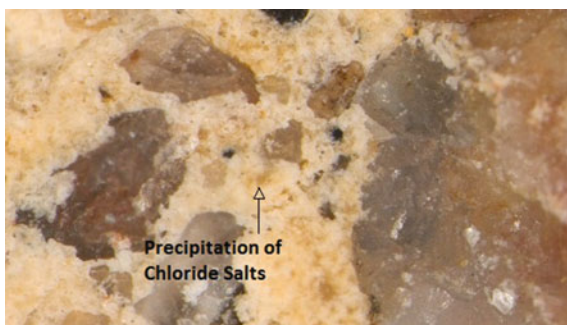
Fig. 5 Stereo microscopic image for BDM particle after 7-day immersion in hydrochloric acid (5% v/v) solution at 2.5× magnification
