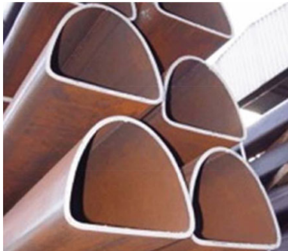
Fig. 1 Semi-elliptical hollow section (Silvestre et al. [13])
