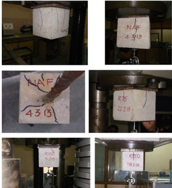
Fig. 2 Observed crack pattern on specimens after pull out test
