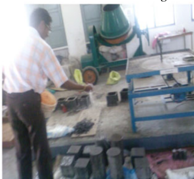
b. Sprinkler curing
