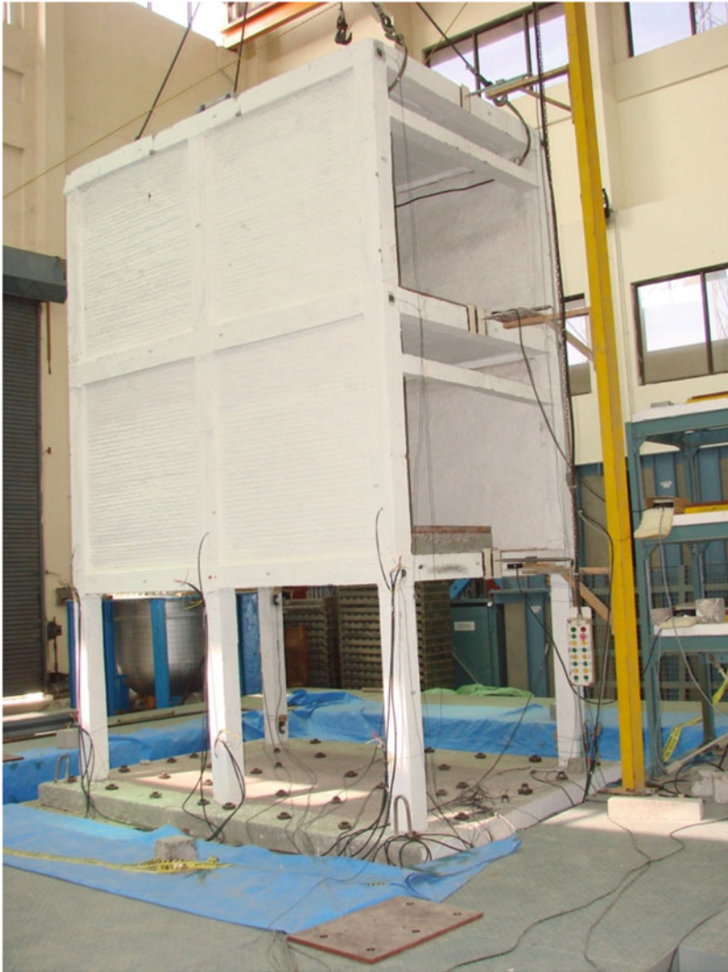
Fig. 1 Shake table test of OGS model frame
