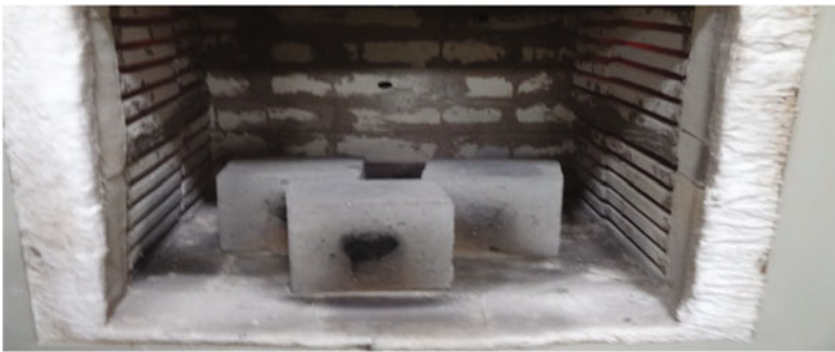
Fig. 5 Specimens kept in an electric furnace
