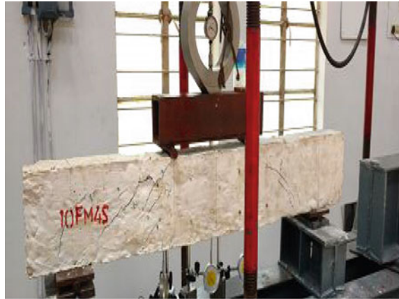
Typical crack pattern of shear beam with fibres -10M4
