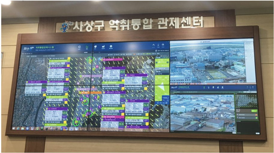
Fig. 2. Sasang IOCC central dashboard showing wind direction and speed, major sources of odor emission, CCTV view of factories. Source: Picture taken by author
