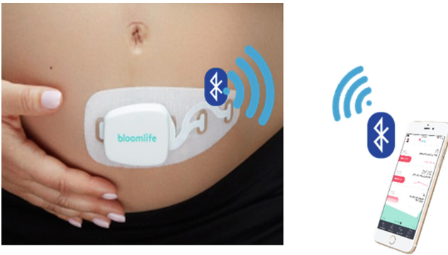
Fig. 1. Technology concept of uterine EMG based pre-term birth monitoring
