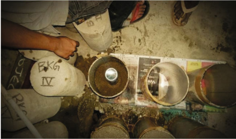
Fig. 3 Casting of cylinders
