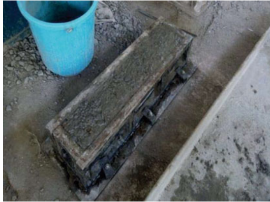
Fig. 6 Specimen after filling and compaction
