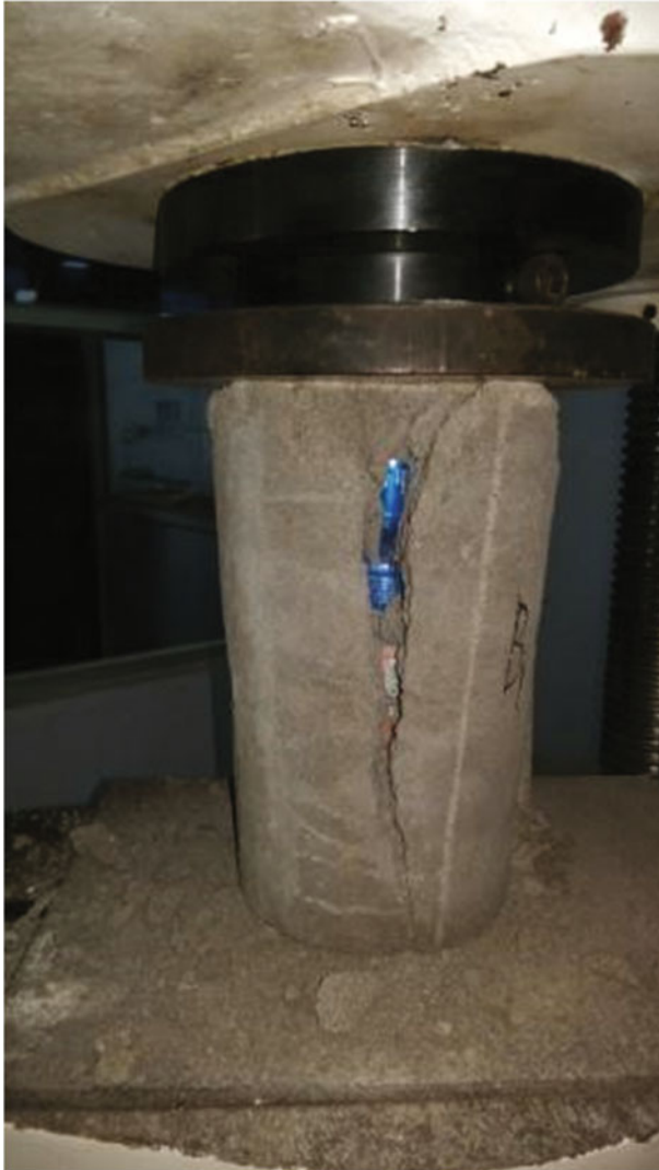
Fig. 4 Failure occur in cylinder
