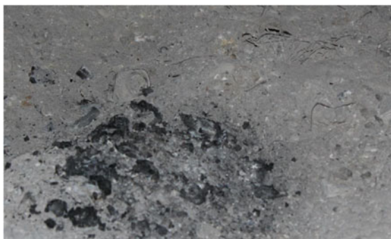
Fig. 1 Residues collected at the bottom of biomedical waste incinerator
