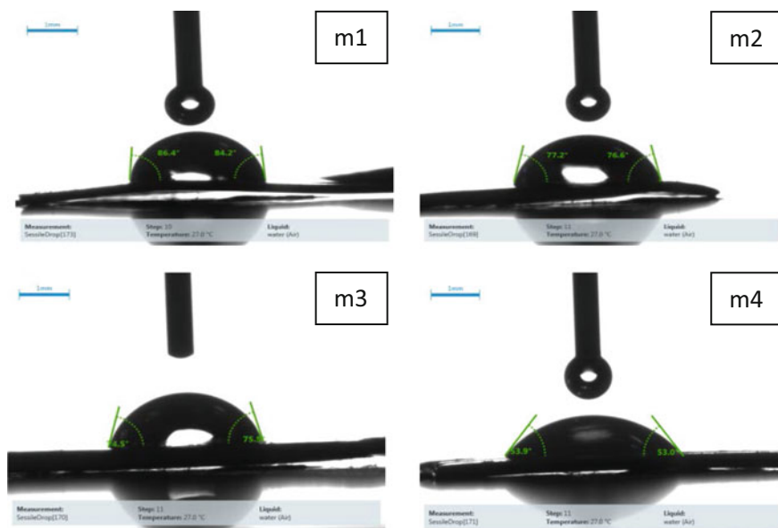
Fig. 5 Images of contact angles for membrane m1, m2, m3, and m4
