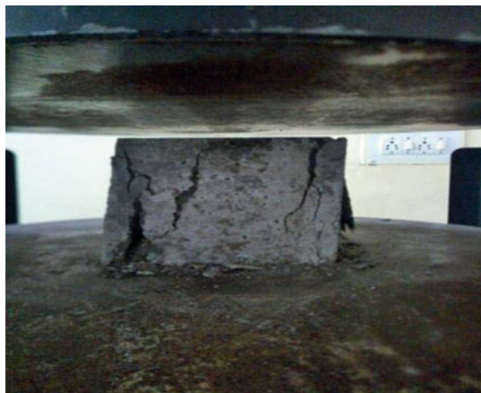
Fig. 7 Gradual failure under compression
