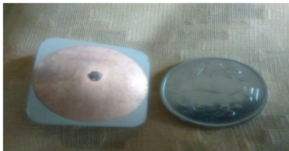
Fig. 6 Fabricated cuff button antenna structure
