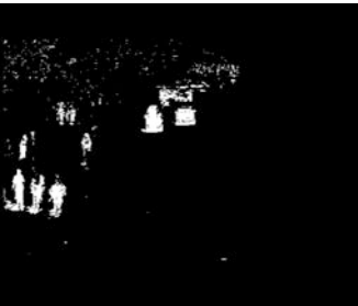
Fig. 5 Output after GMM (noisy frame)
