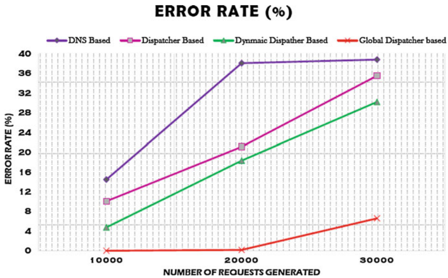
Fig. 5 Comparative analysis of error rate (%) with the proposed GDLB approach
