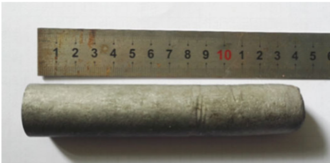
Fig. 12 Tungsten rod after hydrostatic extrusion
