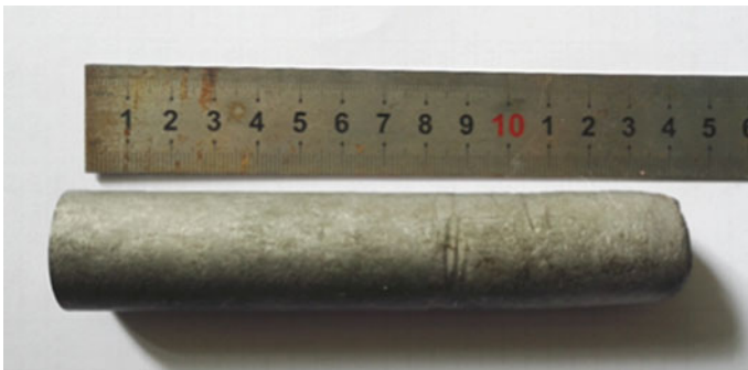
Fig. 12 Tungsten rod after hydrostatic extrusion
