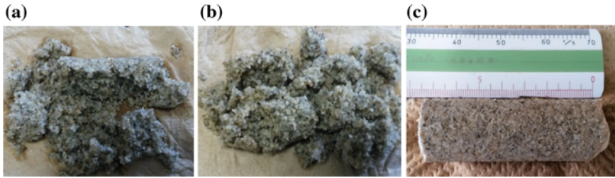
Fig. 5 Appearance of syringe test specimens after 14 days of curing time: a 0.7 M \text{CaCl}_2 + urea, no urease b 0.7 M \text{CaCl}_2 + urease, 3.912 U/mL, no urea, and c 0.7 M \text{CaCl}_2 + urea +urease, 3.912 U/mL
