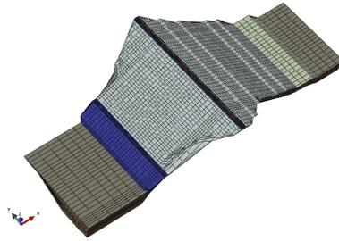
**Fig. 1.** The three-dimensional finite element mesh of dam body.
