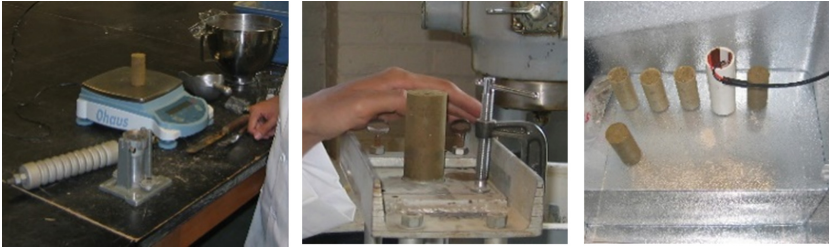
Fig. 3. Preparation of soil specimen
