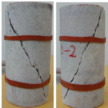
Fig. 5. Failure rock sample including macro sliding surface and axial crack.
