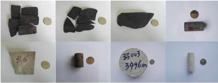
Fig. 1. Examples of rock sample materials for shearing tests. From left to right, from top to bottom: Longmaxi Shale-1, Longmaxi Shale-2, Longmaxi Shale-3, Xuwu Shale, Ordos Sandstone, Junggar Sandstone-1, Junggar Sandstone-2 and Shengli Sandstone.
