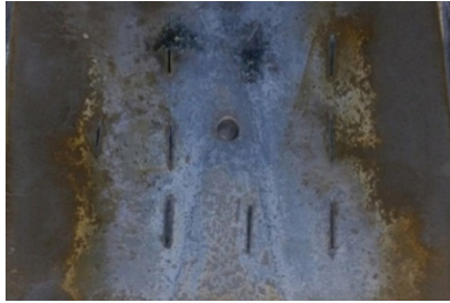
Fig. 8. Healing effectiveness of tunnel segment of experiment two in 50 days
