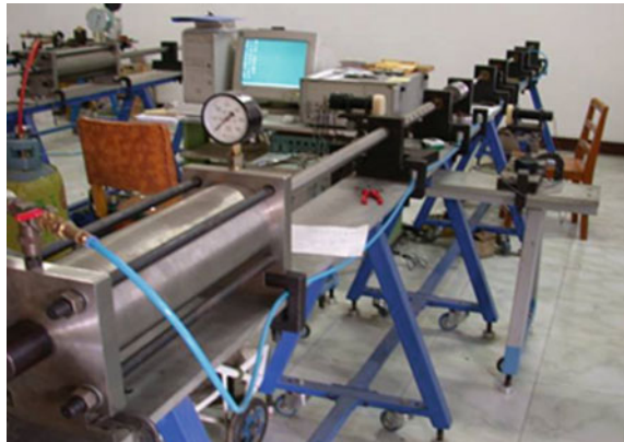
Fig. 4 SHPB equipment for the test of dynamic compressive strength of C/Al 2 O 3 composites
