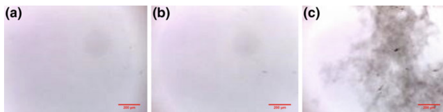
Fig. 6 Optical microscope of the sample. a untreated b added dispersant c added to PAN
