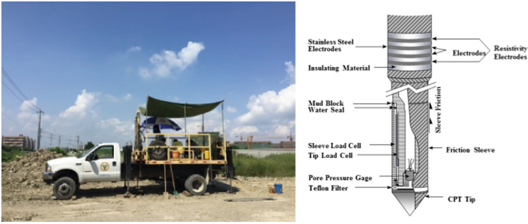
Fig. 2. Schematic diagram of field RCPTU test
