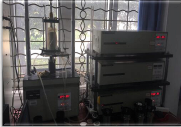
Fig. 1. SLB-1 stress-strain tri-axial shear apparatus.
