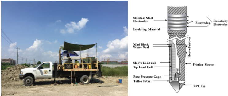
Fig. 2. Schematic diagram of field RCPTU test
