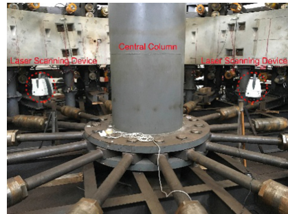
Fig. 11. Placement of two Leica laser scanning devices
