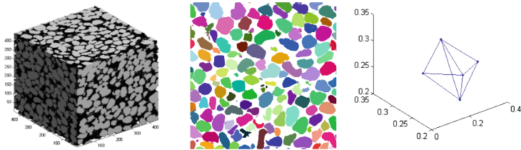
Fig. 2. (a) The 3D structure reconstructed by the CT images serial. (b) One sliced layer after segmentation. (c) Two sample tetrahedron produced by Delaunay tessellation.
