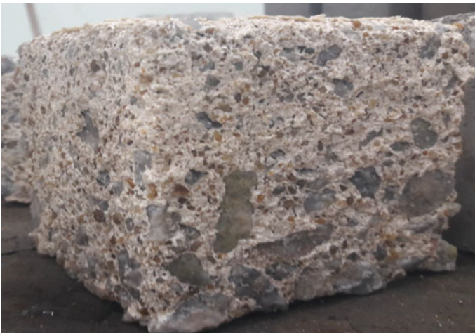
Fig. 3 Eggshell concrete after submerged in sulphuric acid
