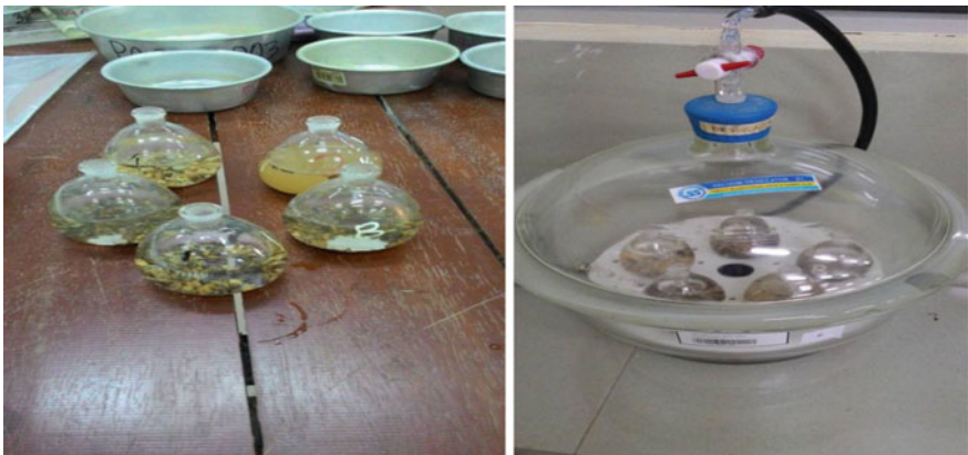
Fig. 4 Equipment and sample used for particle density analysis
