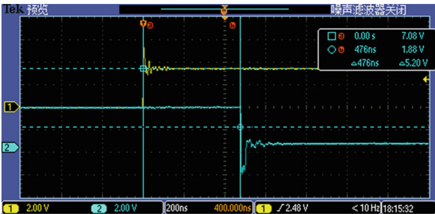
Fig. 7 UM220 OEM plate 1PPS (yellow) and RT2 receiver 1PPS (blue) signal delay
