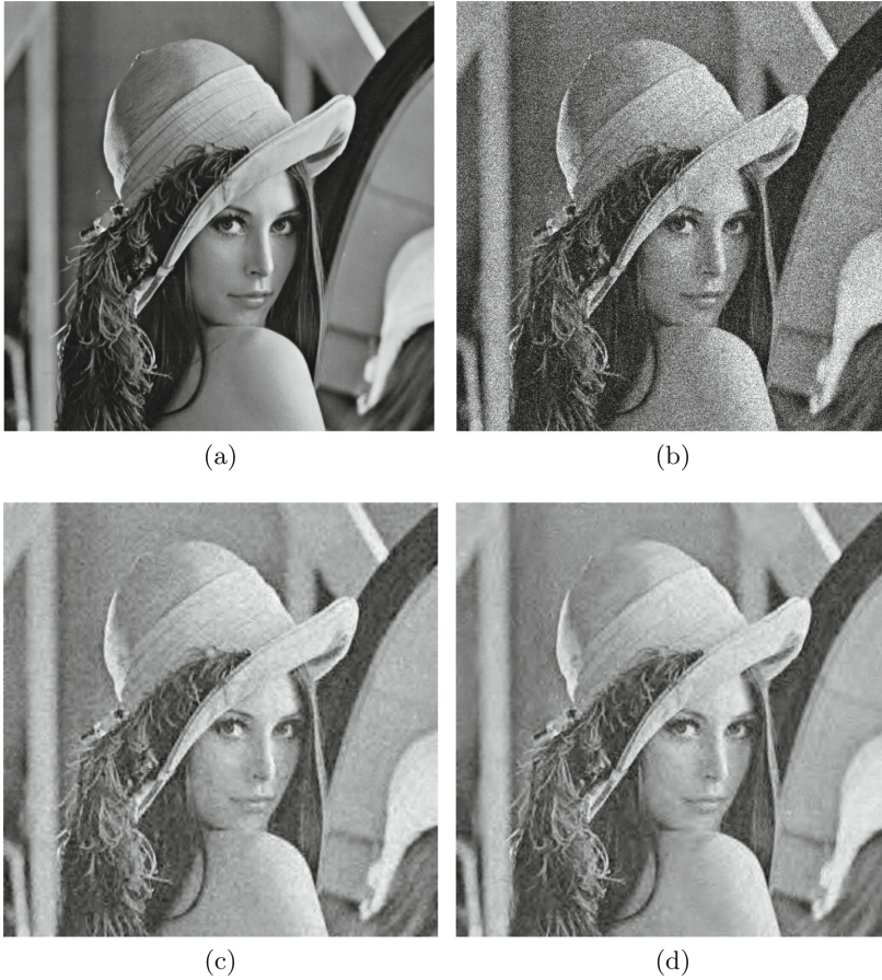
Fig. 4. Image denoising using 2-D DTCWT (a) original image (b) noisy image with \sigma = 30 , PSNR = 18.59 dB. Denoising using (c) Selesnick's 11/13 filters [8], PSNR = 28.73 dB, SSIM [23] = 0.73 and FSIM [24] = 0.90. (d) proposed filters, PSNR = 29.52 dB, SSIM [23] = 0.77 and FSIM [24] = 0.92.
