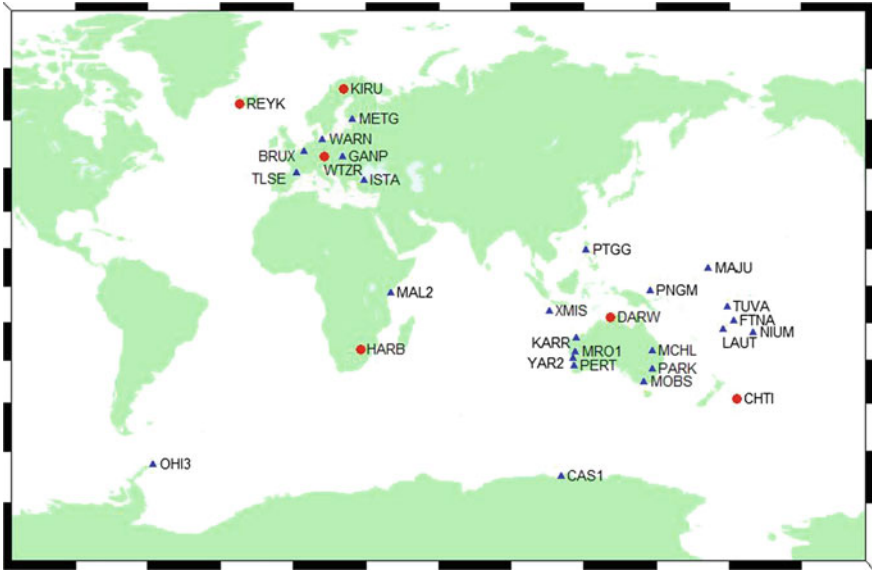
Fig. 1 The distribution of the stations from MGEX (Red dots indicate stations for specific example analysis)
