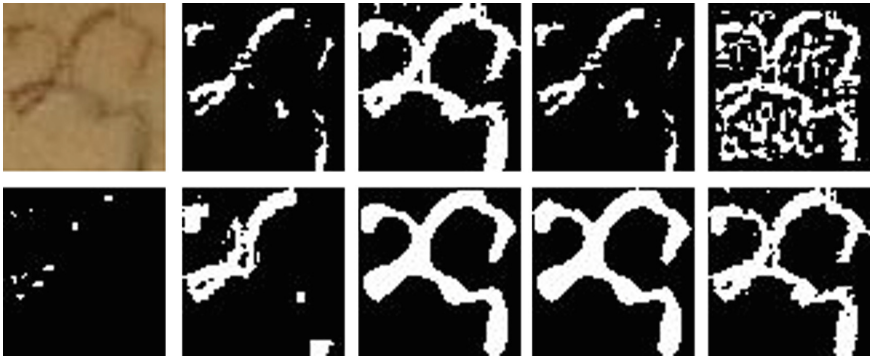
Fig. 4. Segmentation of a sample image from the dataset using different segmentation methods. Top row: Original image, results of Kapur's method, Otsu's method, Kittler's method, and Niblack's method, respectively. Bottom row: Results of Sauvola's method, Su's method, PLT method, NESP method, and MAPS method, respectively.
