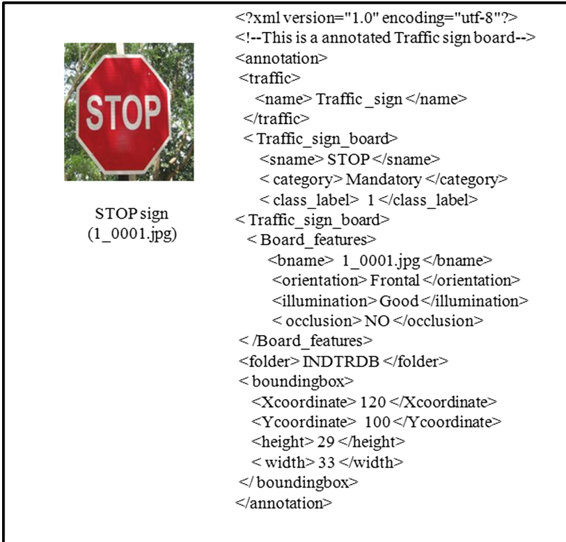
Fig. 4. XML annotation of STOP traffic sign
