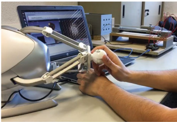
Fig. 3 Novint Falcon, in foreground, with the robotic system and the phantom in background
