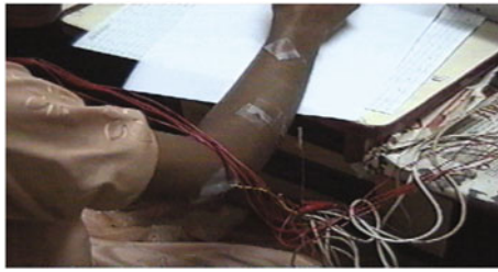
Fig. 6 Subject writing after insertion of micro wire electrodes with indigenous EMG prototype
