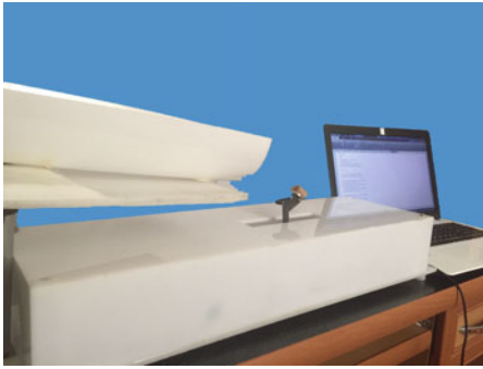
Fig. 1 Front view of the proposed haptic system. The user's forearm and fingertip are located to the hand-arm-rest and the guide respectively and then flexion/extension exercises are produced
