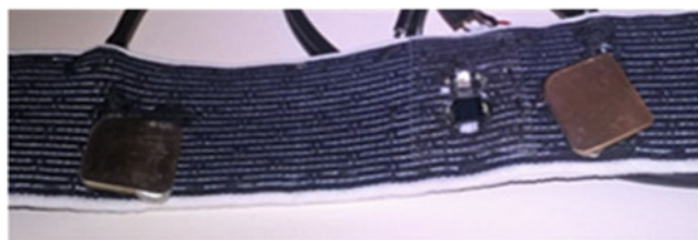
Fig. 1 The rubber belt where were placed measurement parts which are connected directly to the human body and placing of the belt with electrodes and sensors
