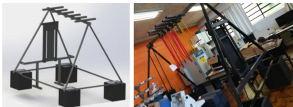
Fig. 1 Prototype of gait system in hypogravity simulation
