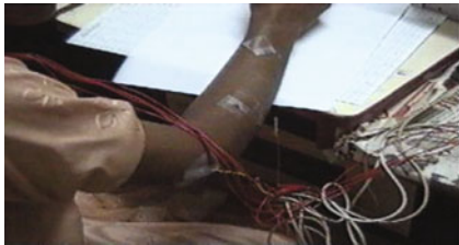
Fig. 3 Subject writing after insertion of micro wire electrodes with indigenous EMG prototype
