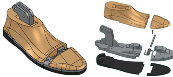
Fig. 3 Novel prosthetic foot 3D model and consisting three basic units: cover, supporting structure, and elastic pad [3]
