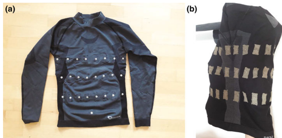
Fig. 1 Experimental garment with integrated textile electrodes: external (a) and internal (b) view
