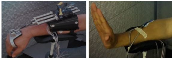
Fig. 2 The setup of the EMG sensors on the forearm, with and without the orthosis
