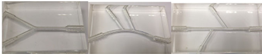
Fig. 2 Flow loop testing for three configurations (Y-shape, Curve, and straight bifurcation. From left to right)
