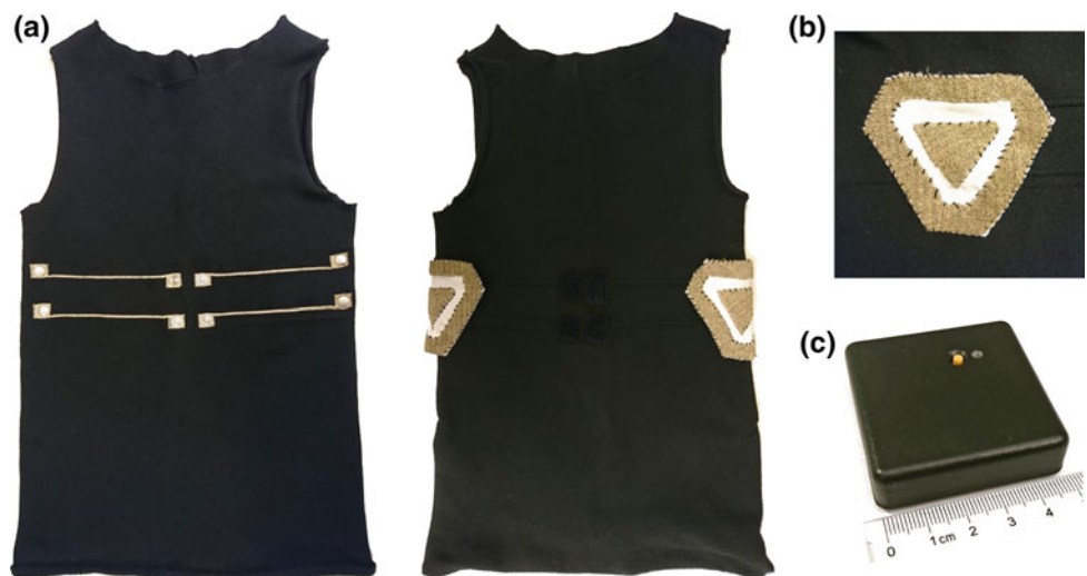
Fig. 1 a The outside (left) and inside (right) of the vest. b The textile electrode pad. c ECGZ2, a compact ECG and electrical bioimpedance measurement device
