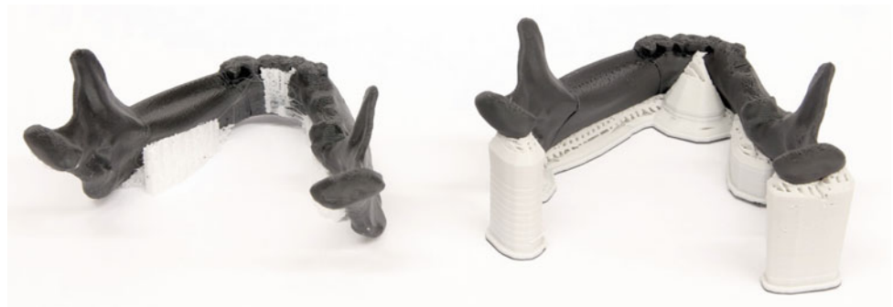
Fig. 3 3D printed jaw templates, Replicator 2X (left), Dimension BST 1200 (right)
