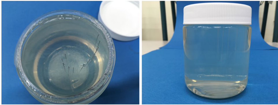
Fig. 1 Needles with a diameter of 0.3 mm, arranged in a projected image not to overlap from the radial direction: left. (This is a prototype, and the number of needles is different from the one used for measurement.) Phantom that removed needle after gelatin solidified: right
