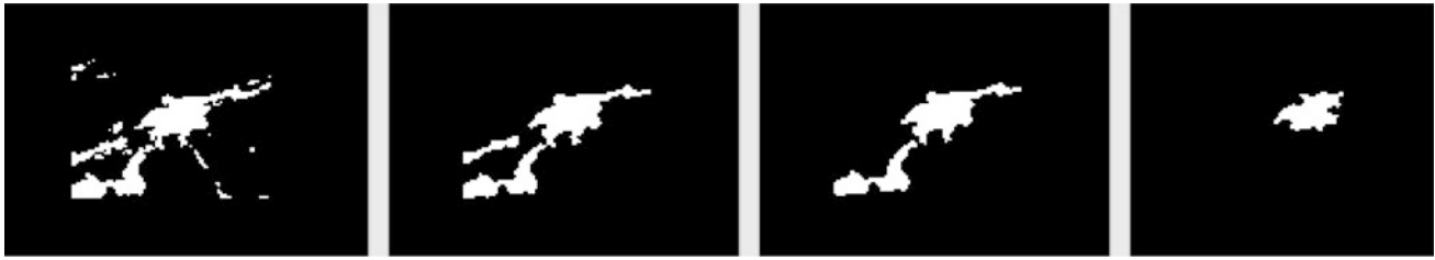
Fig. 3 Results from the different steps of the segmentation algorithm obtained after: (i) thresholding; (ii) morphological processing; (iii) region growing; (iv) interpolation
