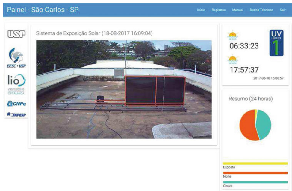
Fig. 2 The automatic solar exposition station for sunglasses installed in the terrace of a building
