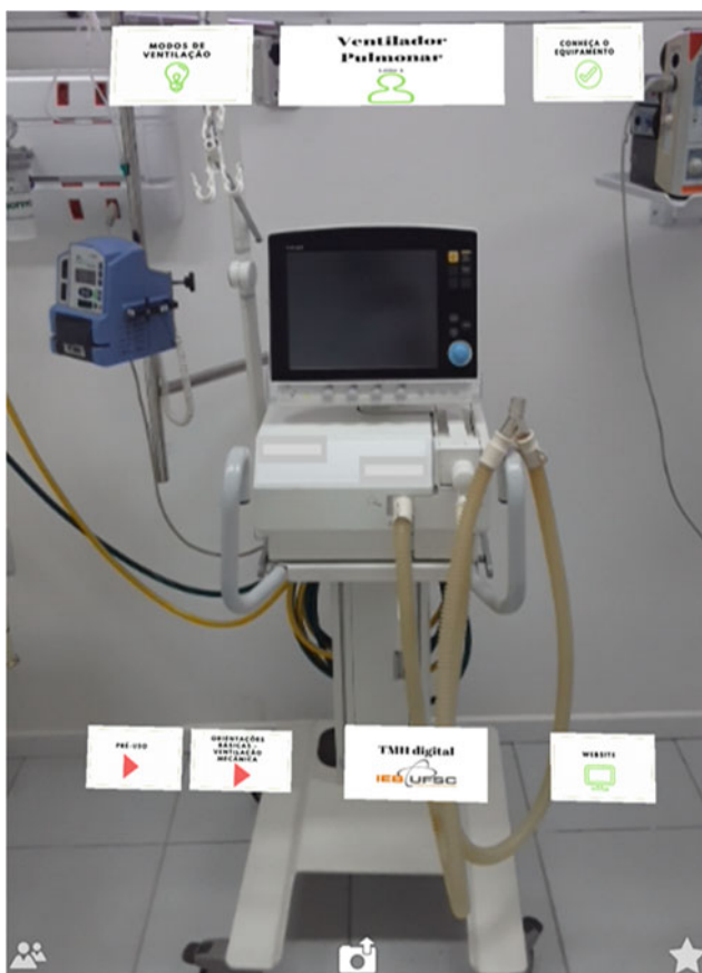
Fig. 3 Prototype of a device running android operational system; this is an example about how the user interact with the technology and how information are presented on the device's screen, when it's camera is pointing and focusing on the medical equipment
