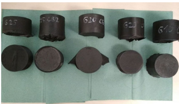
Fig. 1 Some of fabricated samples of human head tissue phantoms
