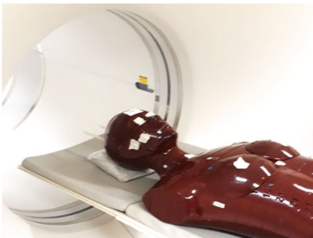
Fig. 2 Positioning of the Alderson female phantom in the gantry
