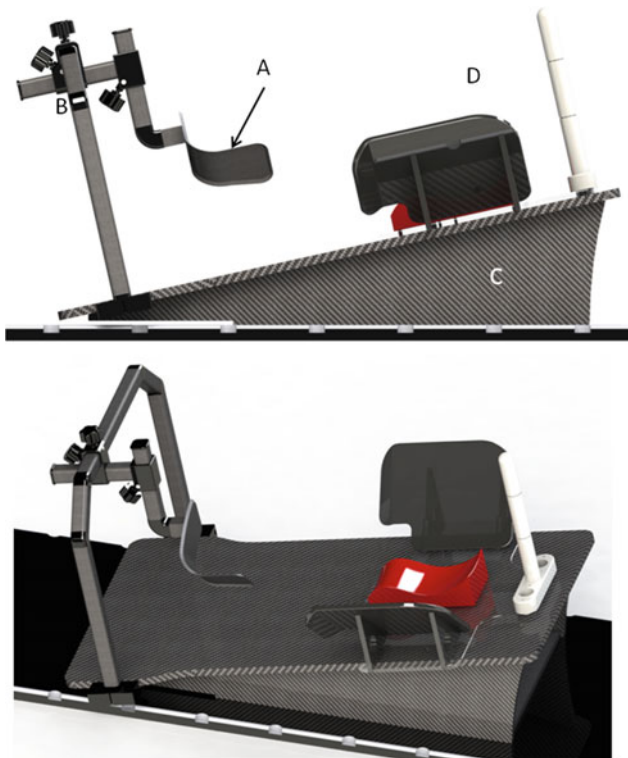
Fig. 1 Lateral and angled views showing: a The carbon fiber breast support “scoop”; b The carbon fibre support frame with Delrin™ joints and locking devices; c Existing supine breast board back support; and d existing head rest, wing-board and hand grip
