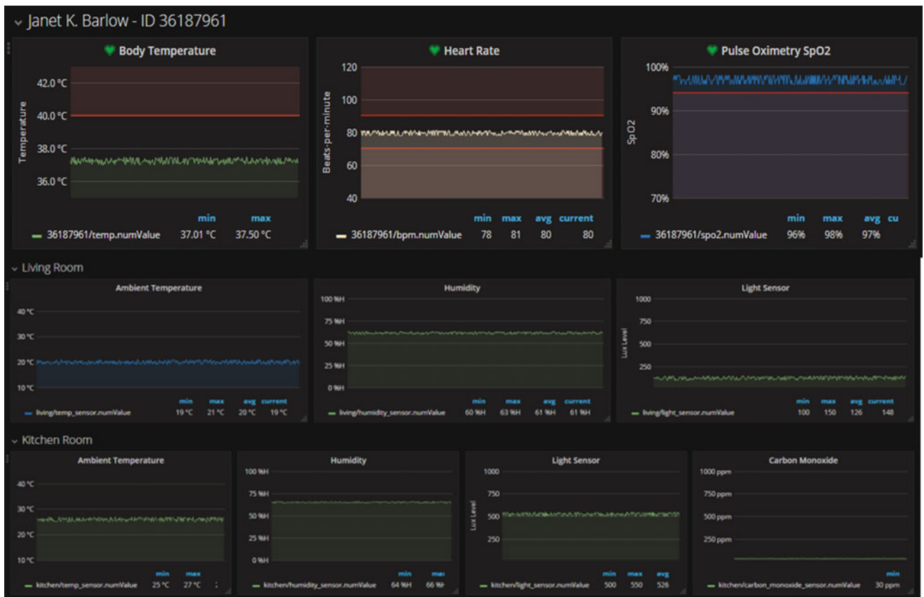
Fig. 8 Up: Real-time graph showing wearable sensors’ values for a specific patient. Down: Real-time graph showing patient’s environment variables
