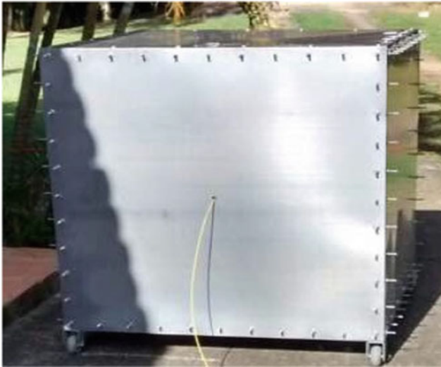
Fig. 1 Cubic structure with aluminum sheets for shielding used for experiments, showing the coaxial cable of the magnetometer
