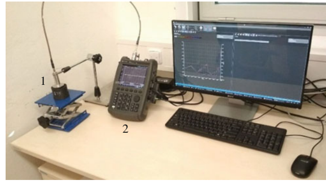
Fig. 2 Experimental setup for measurements of dielectric parameters of fabricated samples, 1—dielectric probe, 2—VNA
