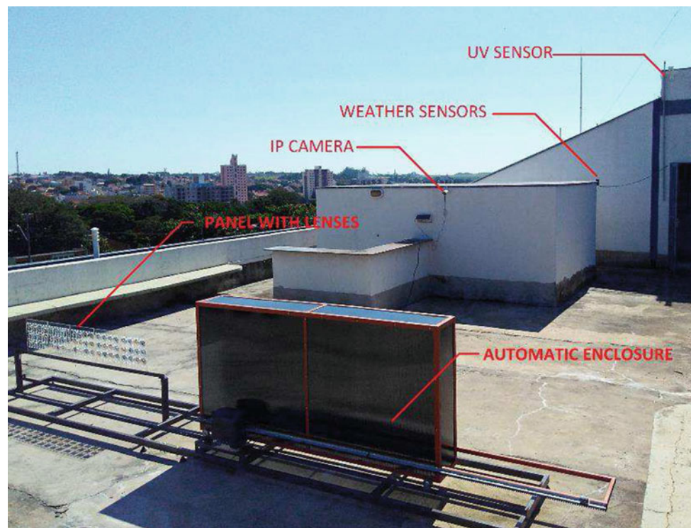
Fig. 1 The automatic solar exposition station for sunglasses installed in the terrace of a building
