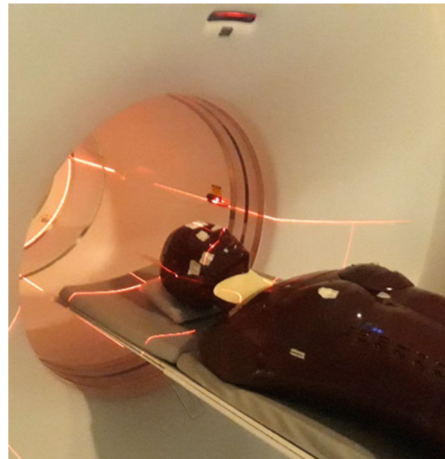
Fig. 3 The phantom Alderson female with the bismuth shielding on the neck spot
