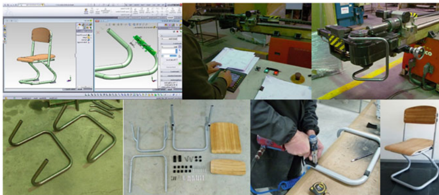
Fig. 19 Example of the production process of one of the prototypes of the Dual_Step Chair
