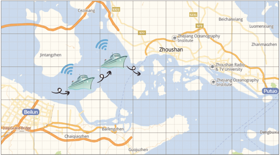
Fig. 2. Trajectory data can be transformed into the grid's data format, which can be imported to the DRN.
