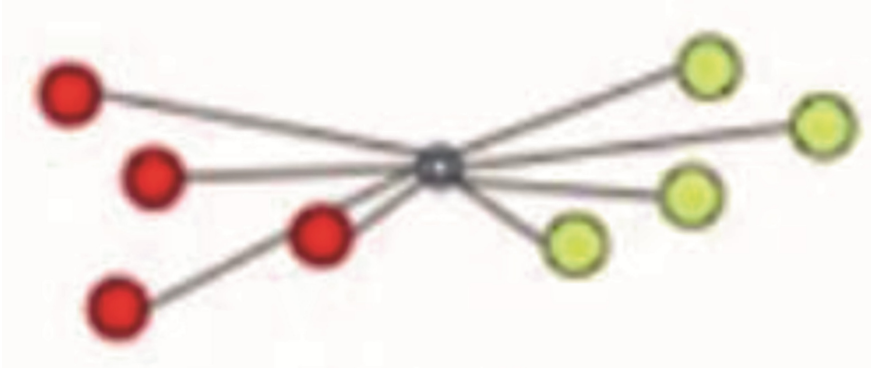
Fig. 6. The log ( AbDi ) which is after data processing. Select all sets from two classes, then calculate the middle point in ( S i , S j ).The distance between each point in the two classes and the center is summed to obtain the distance value between the two classes in this method.
