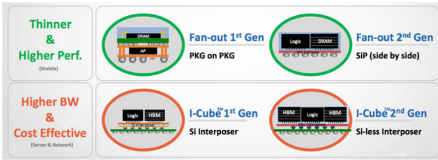
Fig. 8.9 Samsung's next generation packaging technology for housing the AP chipset
