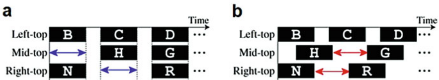
Fig. 22.1 An example of sequence to flash commands in three positions. (a) The conventional method. (b) The proposed method
