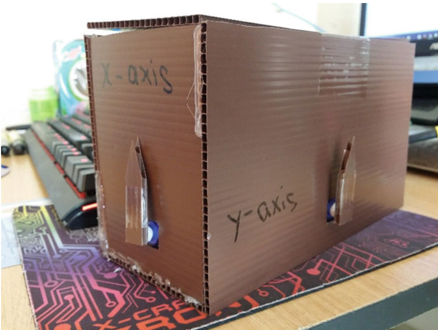
Fig. 9 Position of servo motor when SN-IMU5D-LC is horizontal to the ground
