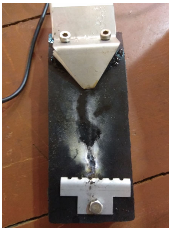
Fig. 3 Carbon formed on the specimen surface
