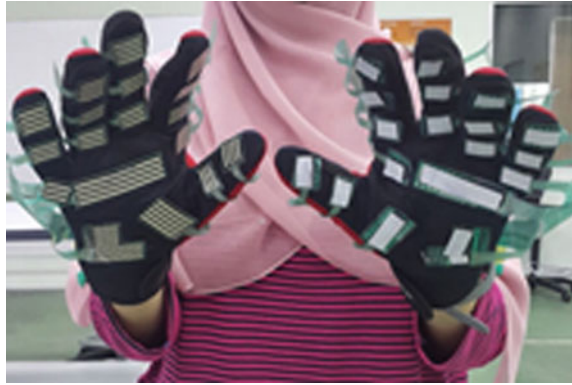
Fig. 3 Grip sensor built-in with glove
