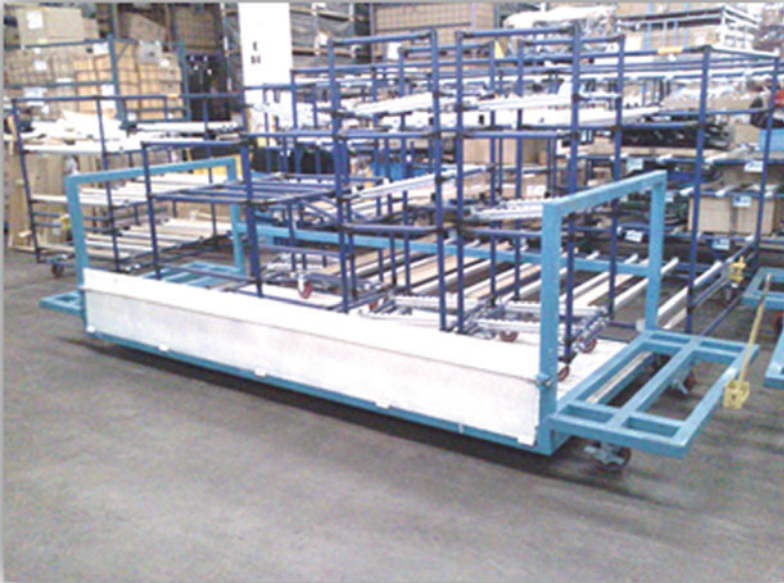
Fig. 3 Mother trolley carry carts in plant layout of actual automation factory
