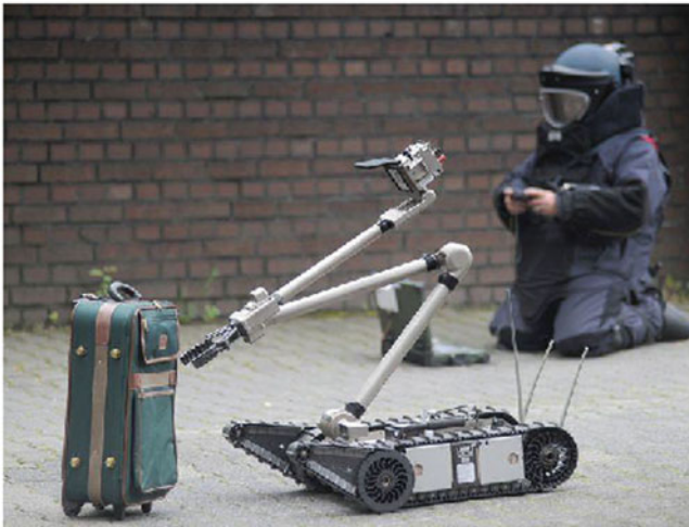
Fig. 1 The interaction of the operator, a bomb squad officer with the remote robotic system, while investigating a suspected explosive device [9]
