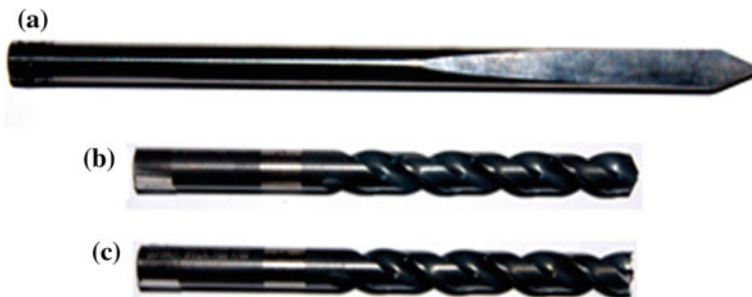
Fig. 2 Drill bits used in the experiments: a dagger drill, b twist drill and c brad drill
