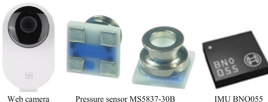
Fig. 16 Camera and sensors equipped to X4-ROV
