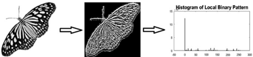
Fig. 4 Gray scaled image being converted to LBP image and LBP histogram
