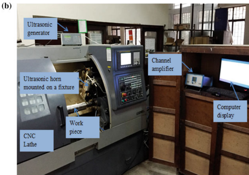
Fig. 12 a Schematic and b actual setup for UAT experimentation (Sharma and Pandey 2016d)
