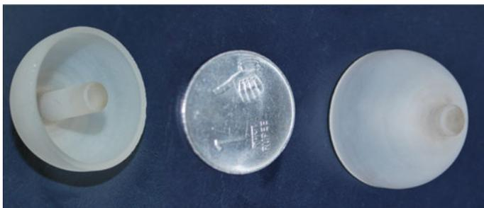
**Fig. 15** Fused silica shell (two different views)
