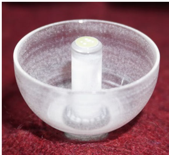
Fig. 18 Hemispherical shell of fused silica after plasma polishing
