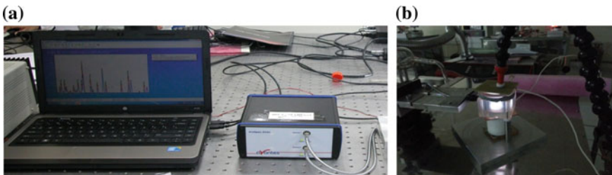
Fig. 12 a Optical emission spectroscopy set up, b its probe positioned at plasma chamber
