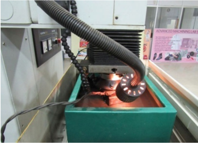
Fig. 2 PMEDM setup (Tripathy and Tripathy 2017b, c)
