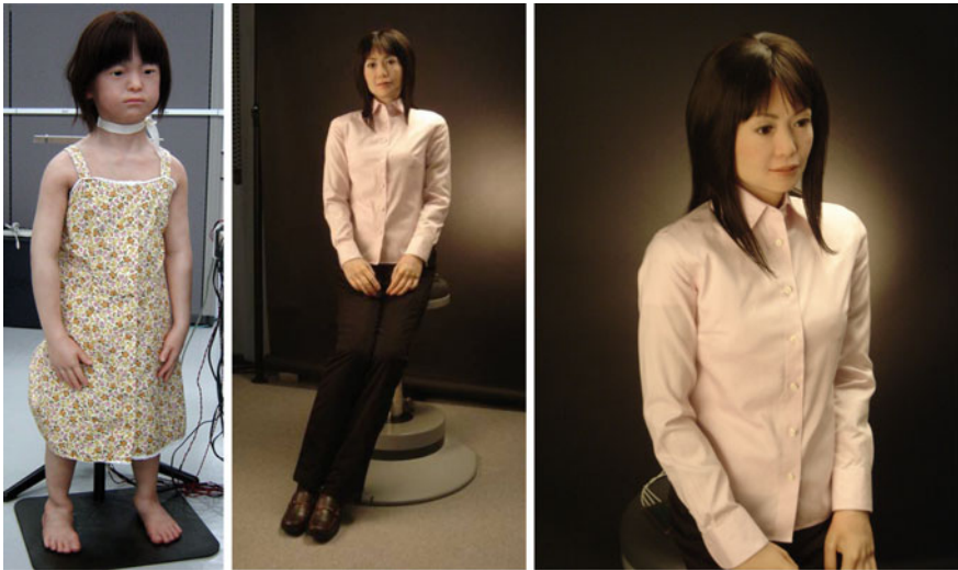
Fig. 2.3 First android, Repliee R1 (left; developed by Osaka University), and the latest android, Repliee Q2 (right; developed by Osaka University and Kokoro Corporation)
