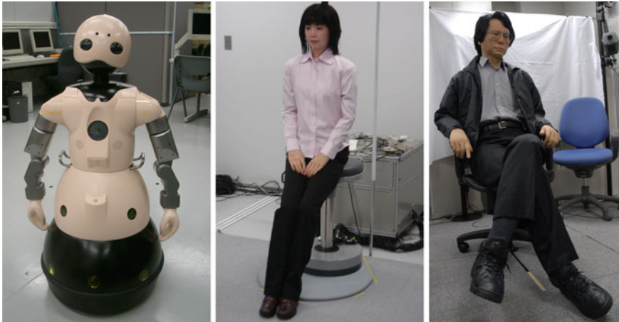
Fig. 2.1 Three categories of humanlike robots: humanoid robot Robovie II (left: developed by ATR Intelligent Robotics and Communication Laboratories), android Repliee Q2 (middle: developed by Osaka University and Kokoro Corporation), geminoid HI-1 (right: developed by ATR Intelligent Robotics and Communication Laboratories)
